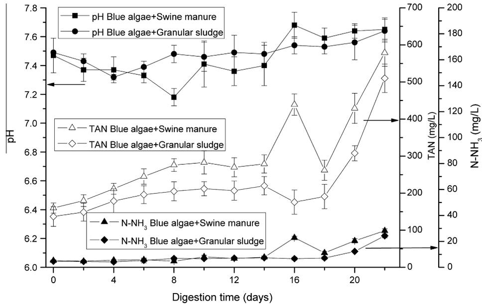
Fig. 2. pH, TAN and  $\text{N-NH}_3$  changes during digestion and codigestion of Taihu blue algae.
