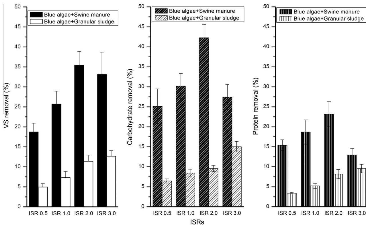
**Fig. 3.** VS, carbohydrate and protein removal rates after digestion and codigestion of Taihu blue algae at different ISRs.
