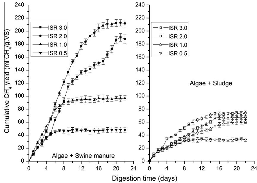
Fig. 1. Cumulative  $\text{CH}_4$  production during batch AD of Taihu blue algae with swine manure and granular sludge at different ISRs.
